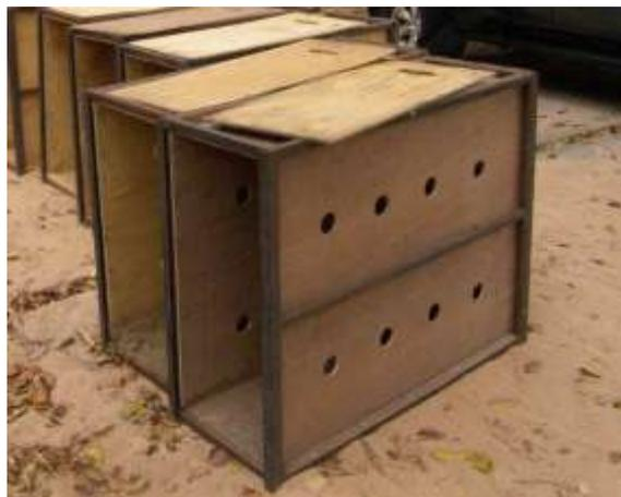
Figure 3: Example of deer box, where the horizontal side braces are also carry handles that don't protrude beyond the width of the box
