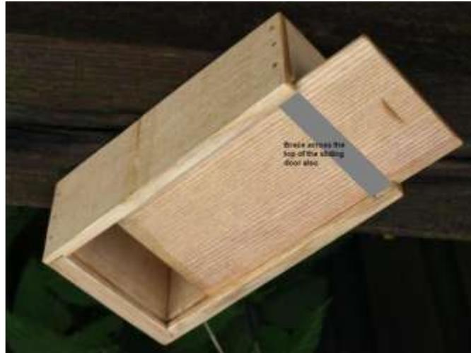
Figure 1: The front and back slide out doors should generally follow this design (with an extra brace where the grey band is)
